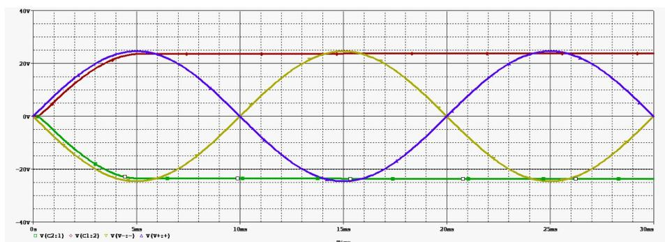
Figure 2.3: Voltages in the PSU without any load.
