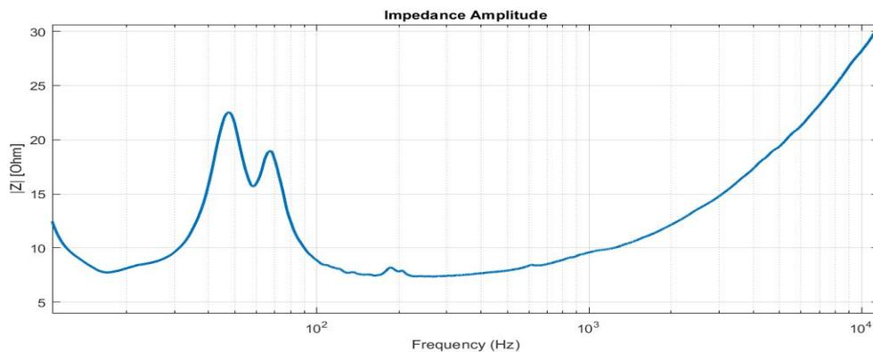
Figure 3.4: Absolute value of the impedance as function of the frequency, for woofer 1.
