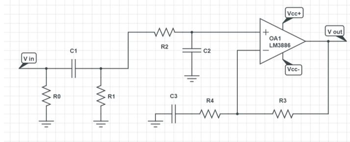
Figure 5.1: Complete amplifier circuit (without mute).
