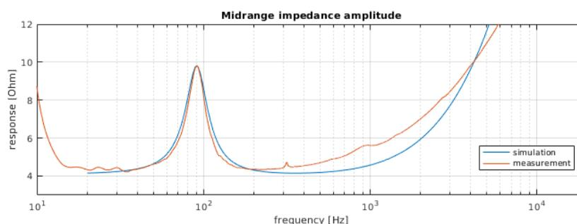
Figure 3.1: Comparison of the impedance measurement and simulation for the midrange driver.
