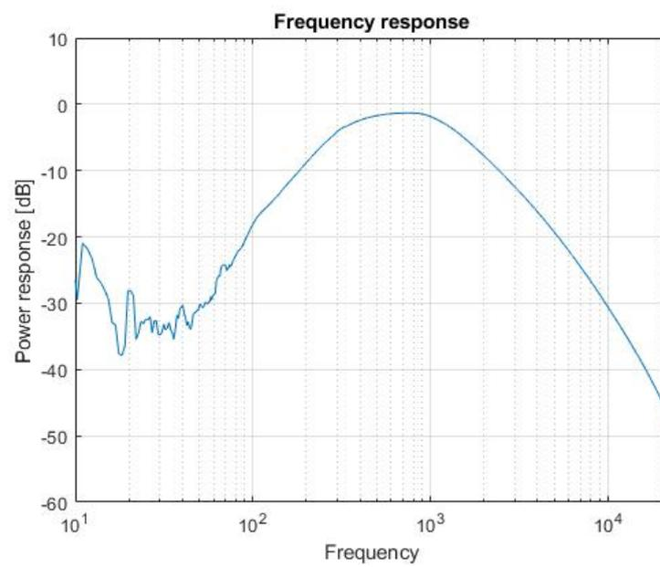
Figure 8.43: Electrical response band-pass filter with Zobel network
