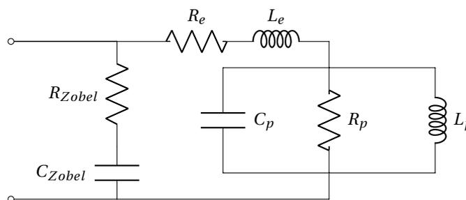
Figure 4.1: Model of a speaker element with Zobel Network
