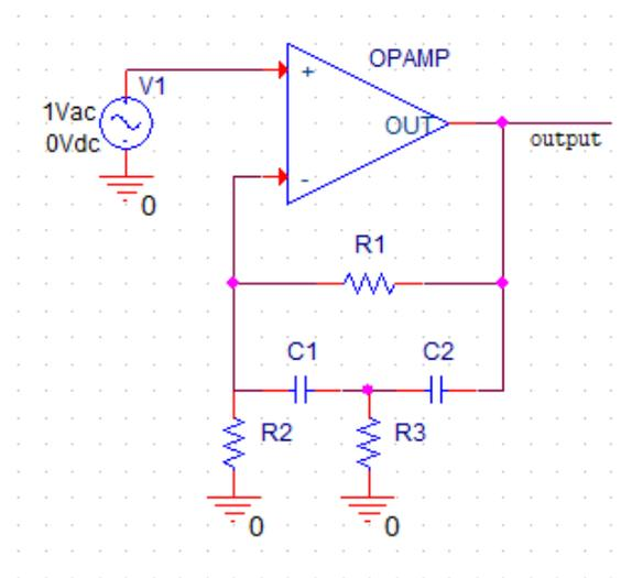
Figure 9.2: OP-AMP with second order high-pass filter in its feedback loop.
