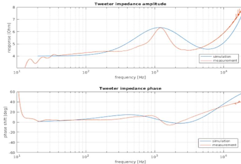
Figure 3.2: Comparison of the simulated and measured impedance amplitude and phase response of the tweeter. Most noticeable are the difference in bandwidth and the difference at high frequencies.
