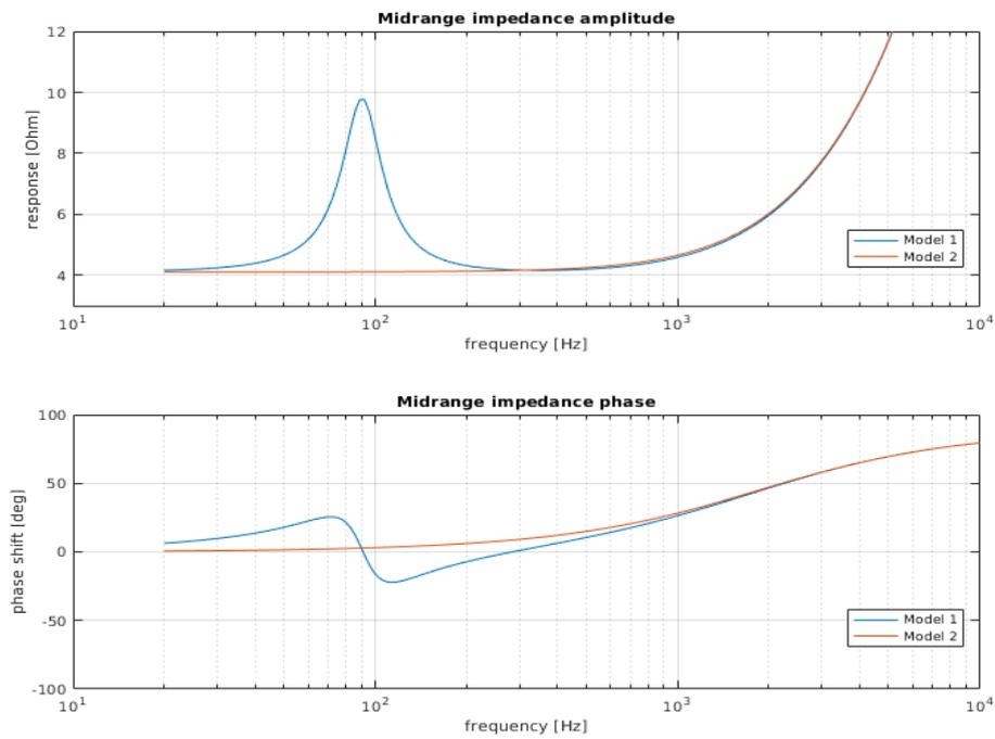
Figure 8.11: Impedance amplitude and phase graphs from the impedance simulation of the midrange speaker driver, comparing model 1 and model 2.
