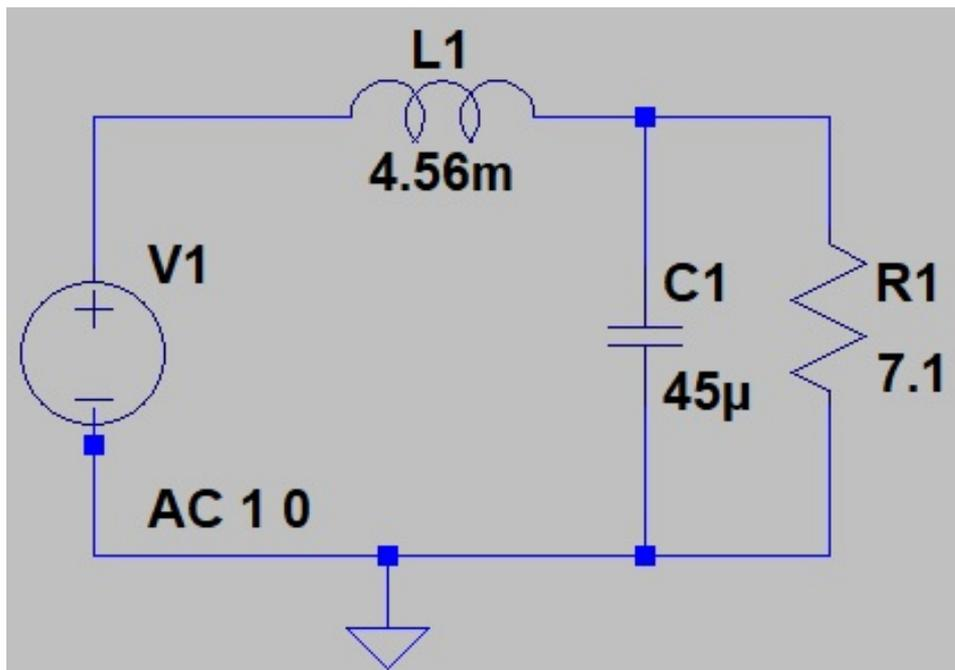
Figure 8.30: Low pass filter circuit
