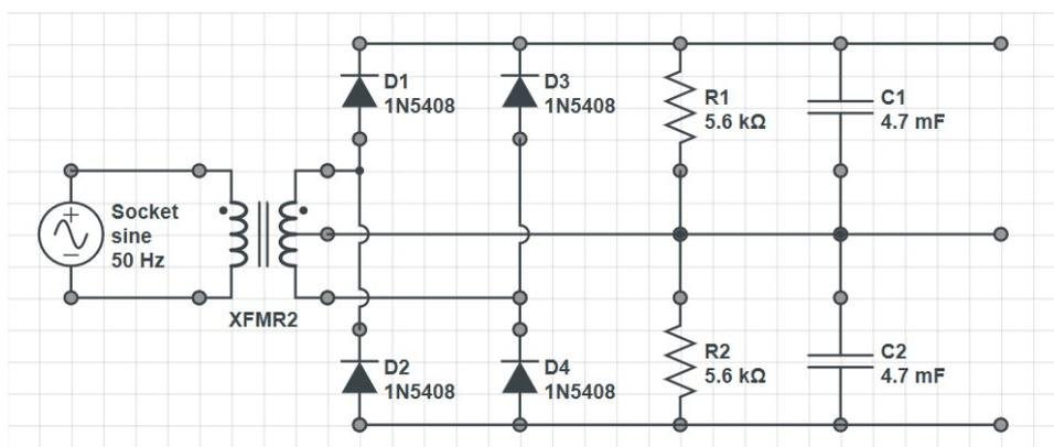
Figure 2.1: Power supply schematic.
