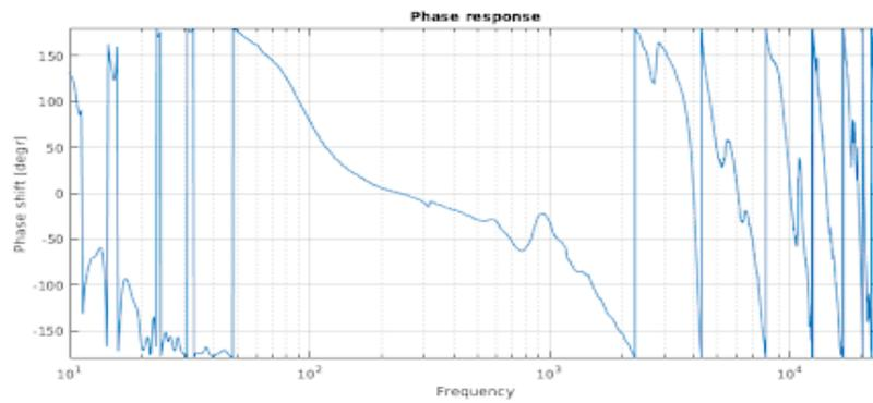
Figure 8.19: Acoustical phase response of the midrange driver.
