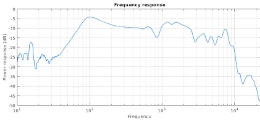
Figure 8.15: Acoustical frequency response of the midrange driver.
