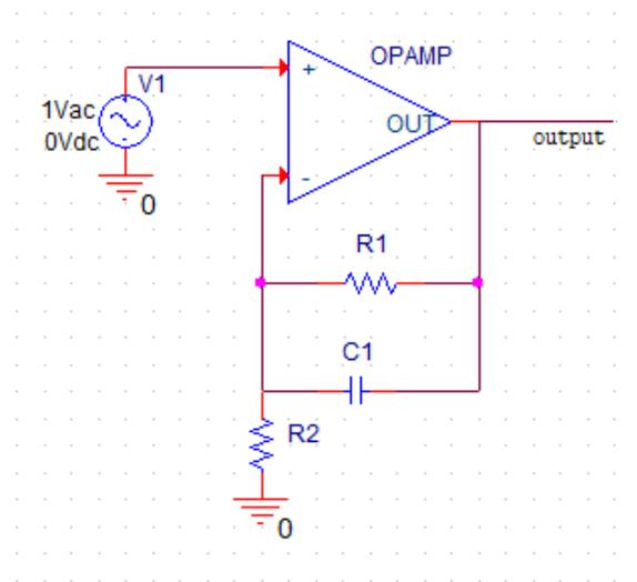
Figure 9.1: OP-AMP with first order high-pass filter in its feedback loop.
