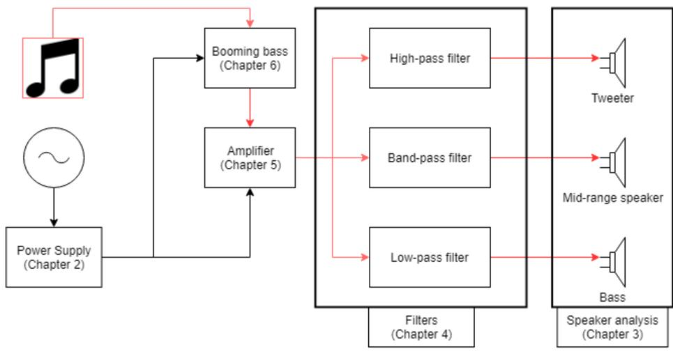
Figure 1.1: Block diagram of the audio system.
