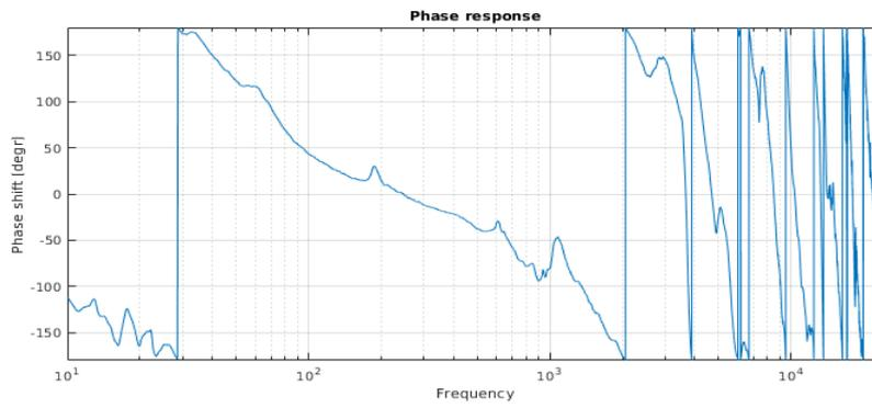
Figure 8.21: Acoustical phase response of woofer 1
