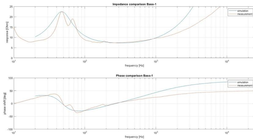
Figure 8.13: Comparison of measured and simulated impedance amplitude and phase of woofer 1
