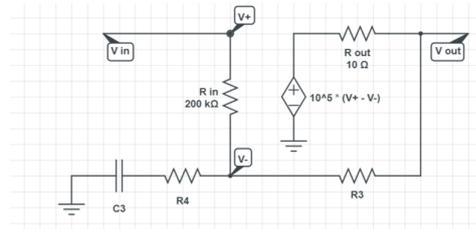
Figure 5.3: Real op-amp circuit.
