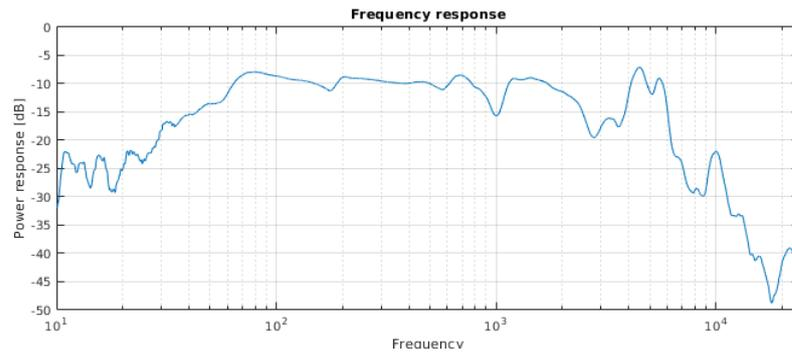
Figure 8.17: Acoustical frequency response of woofer 1
