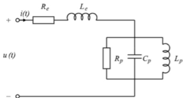
Figure 8.6: Simplified impedance model for a speaker element.
