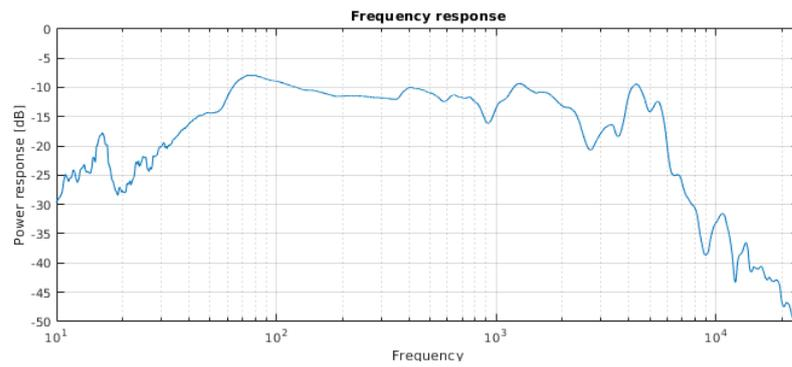
Figure 8.18: Acoustical frequency response of woofer 2
