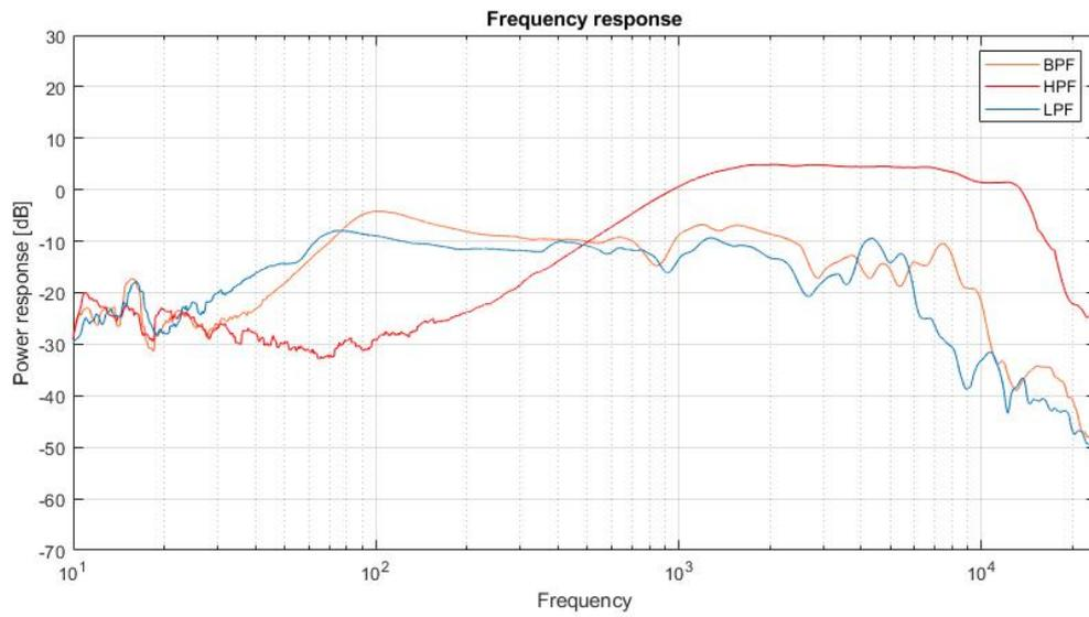
Figure 8.29: Frequency-response measurement Woofer
