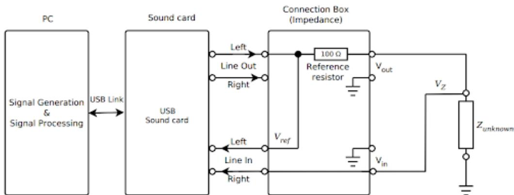
Figure 8.8: Measurement setup for measuring an unknown impedance. [?, figure 14.10, p. 146]
