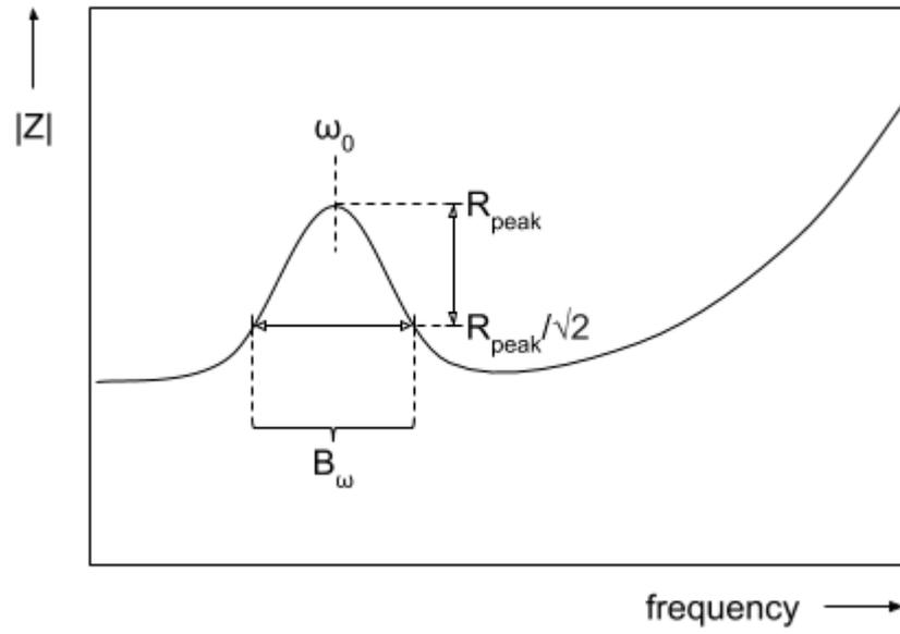
Figure 8.10: Typical impedance amplitude graph from a measurement, showing important parameters.
