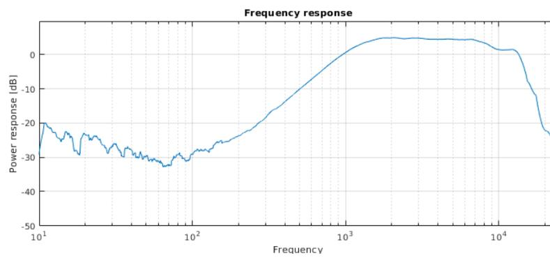
Figure 8.16: Acoustical frequency response of the tweeter
