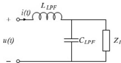
Figure 4.2: A model of a second order Low-pass filter
