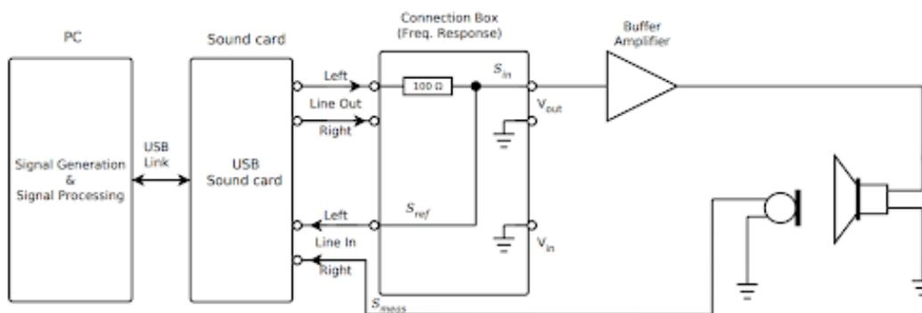
Figure 8.9: measurement setup for short distance acoustic measurement. [?, figure 15.5, p. 153]
