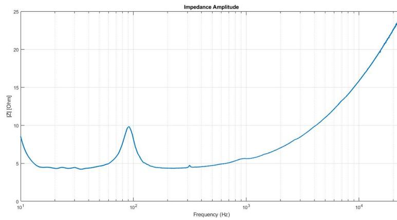
Figure 8.27: Impedance measurement Midtuner
