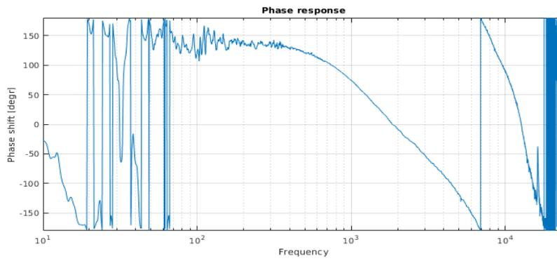
Figure 8.20: Acoustical phase response of the tweeter
