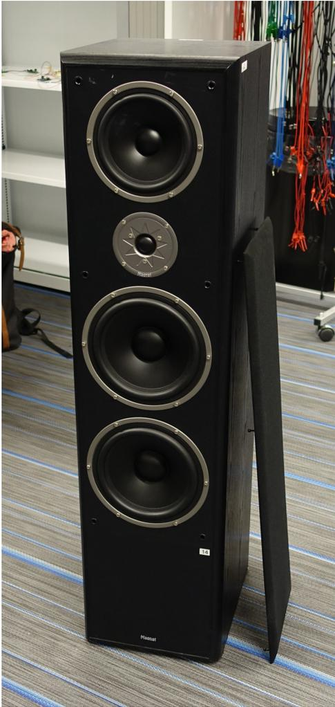
Figure 8.3: The speaker we received. The four speaker drivers can be seen, from top to bottom: the midrange driver, tweeter, woofer 1 and woofer 2.
