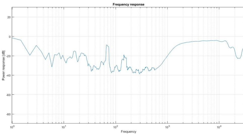
Figure 8.45: Near field acoustic transfer high-pass filter
