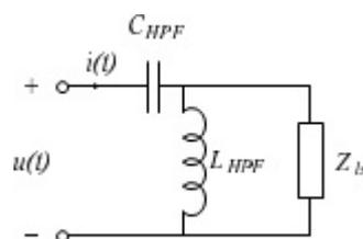
Figure 4.3: A model of a second order High-pass filter
