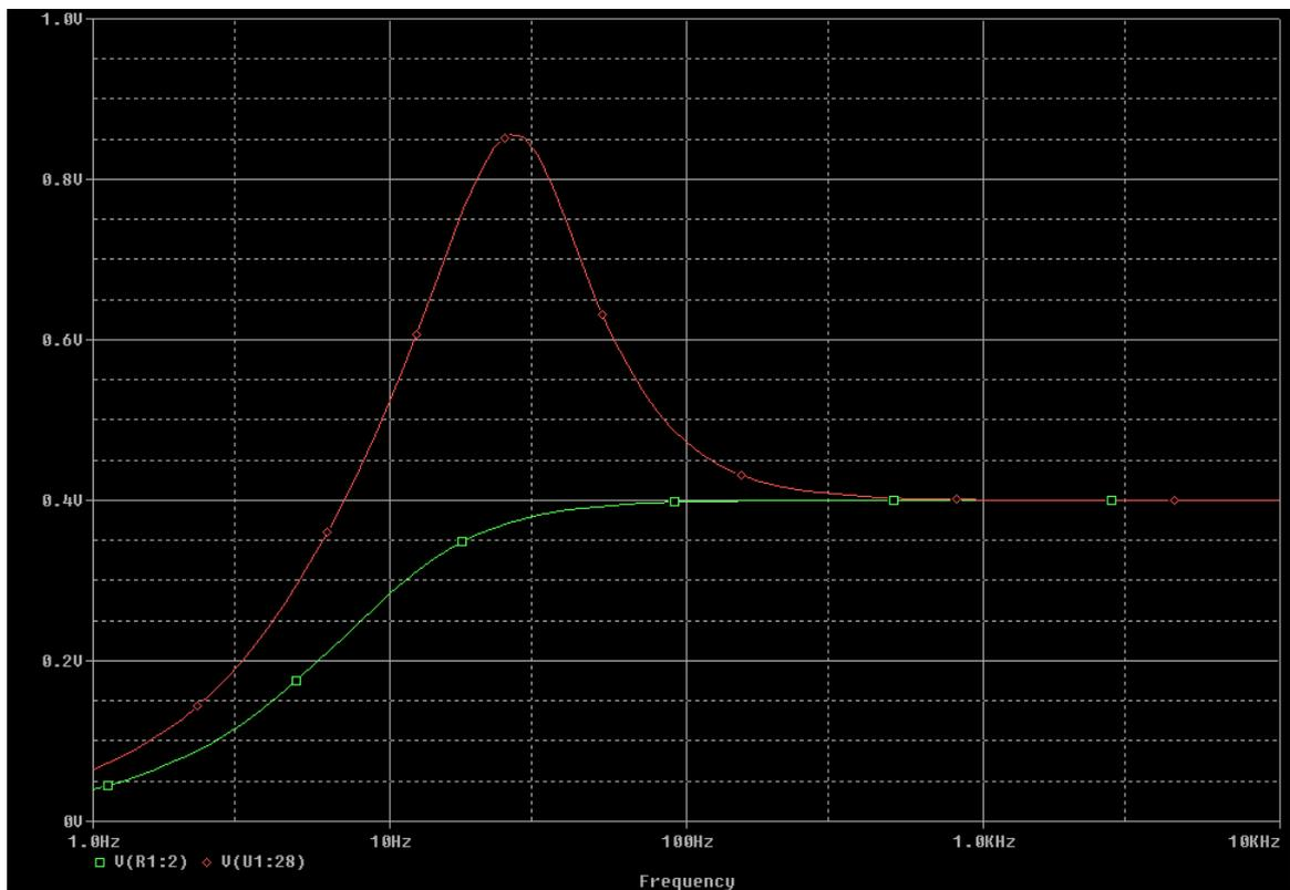
Figure 9.4: OP-AMP with second order high-pass filter in its feedback loop.
