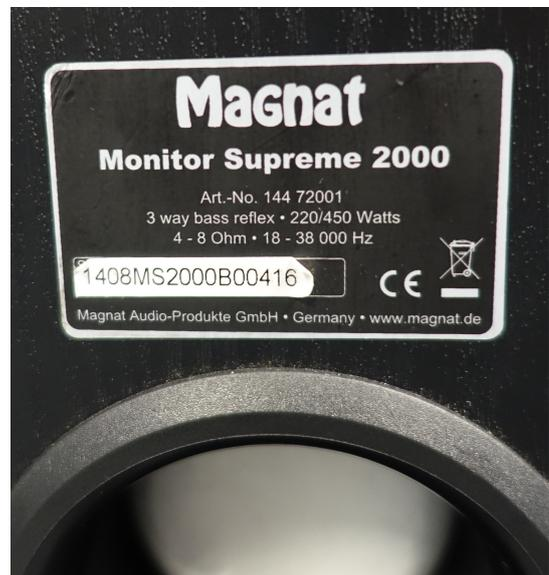
Figure 8.4: The type plaque on the back side of the speaker. Underneath it, the upper bass reflex duct is visible with a Styrofoam ball stuffed in it.
