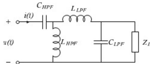
Figure 4.4: A model of a second order Band-pass filter
