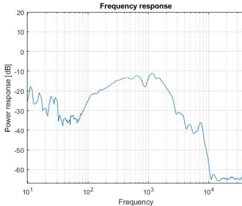
Figure 8.46: Near field acoustic transfer band-pass filter
