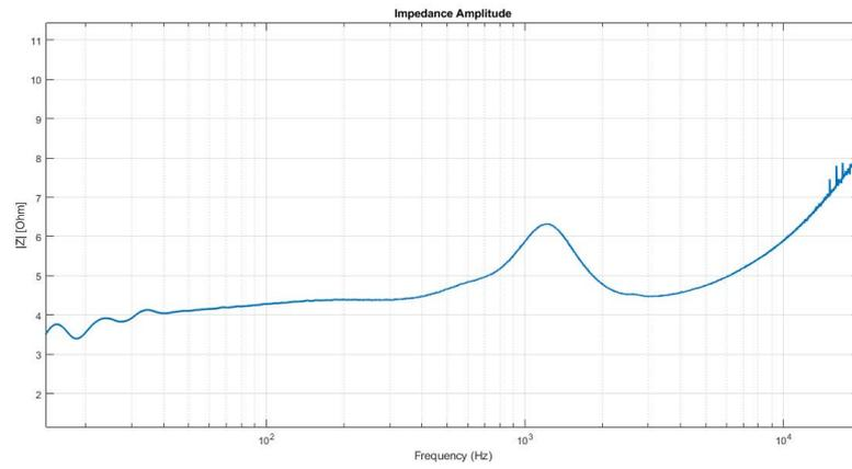
Figure 8.28: Impedance measurement Tweeter
