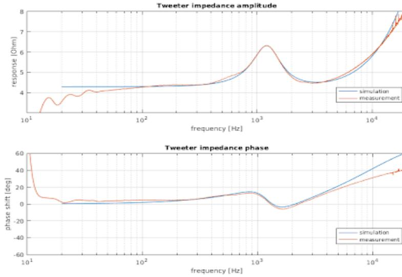
Figure 3.3: Comparison of the measured impedance amplitude and phase response of the tweeter and the adjusted simulation.
