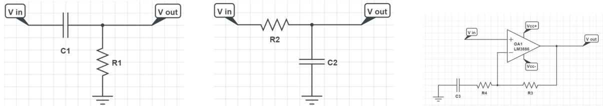
Figure 5.2: (from left to right) High-pass filter, Low-pass filter, Amplifier with high-pass filter.
