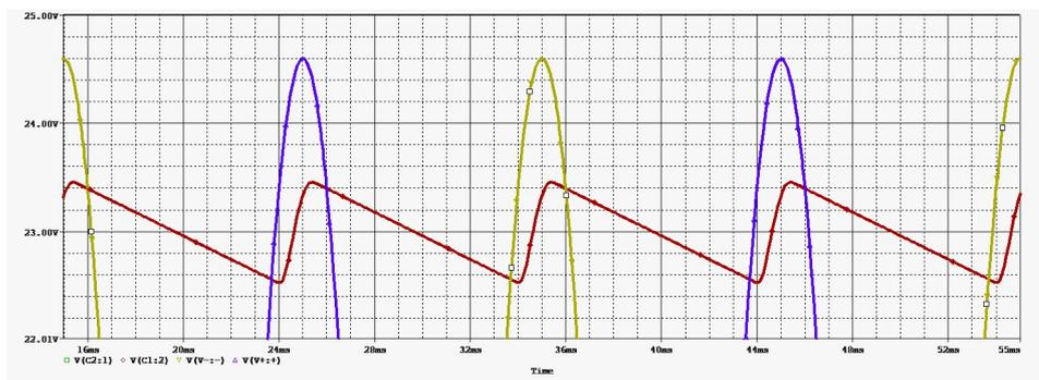
Figure 2.4: Ripple voltage at the positive terminal with a load of 1 Amp.
