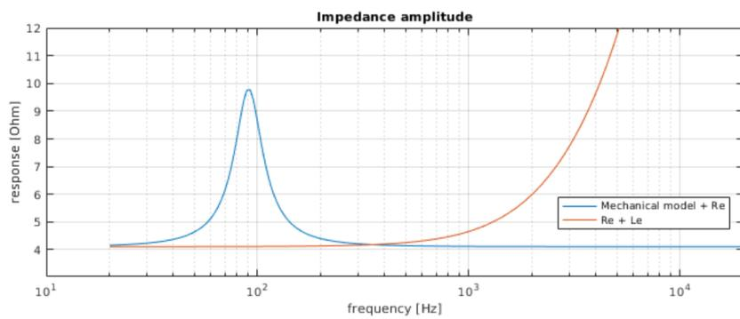
Figure 8.12: The combined impedance from the mechanical model approaches zero and the impedance from the self-inductance  $L_e$  increases significantly above the resonance frequency. This simulation was made using the values for the midrange driver.
