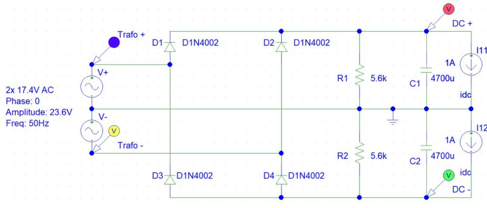
Figure 2.2: Schematic used for simulation under loaded condition.
