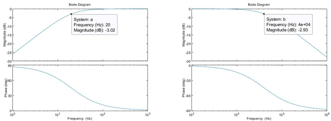
Figure 8.49: (from left to right) Bode plot of high-pass filter, Bode plot of low-pass filter
