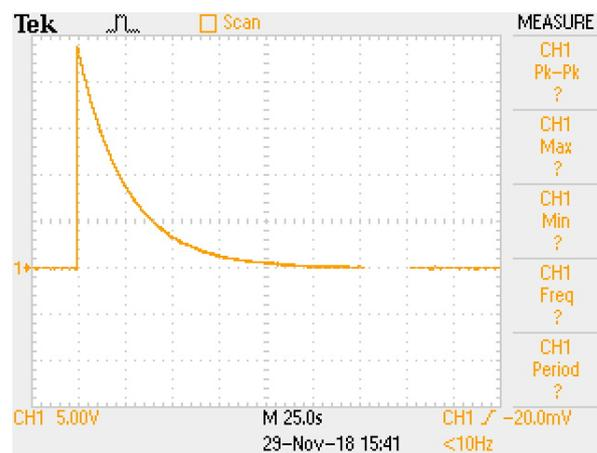
Figure 8.2: Discharging of the capacitor at the positive terminal.
