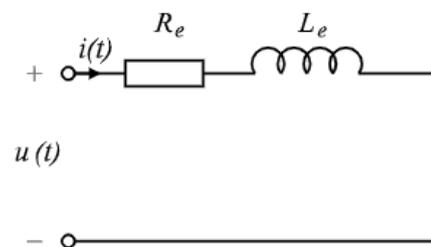
Figure 8.7: Simplified impedance model for frequencies above the resonant frequency.
