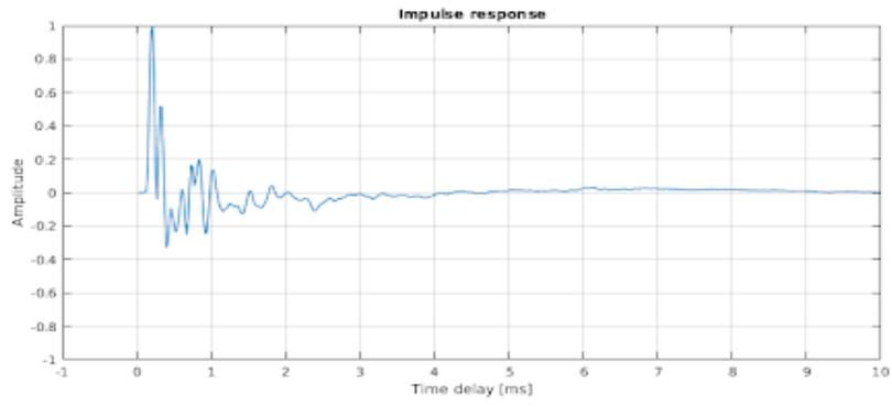
Figure 8.23: Impulse response of the midrange driver.
