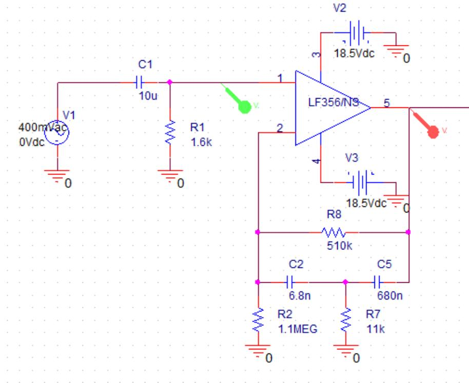
Figure 9.3: OP-AMP with second order high-pass filter in its feedback loop.
