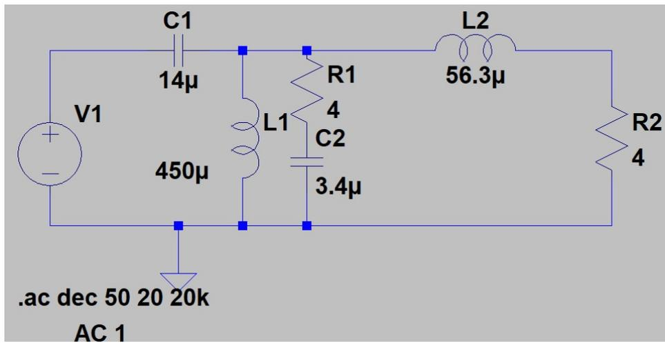
Figure 8.34: High pass filter circuit
