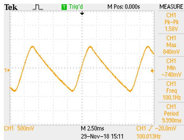
Figure 8.1: Measured ripple voltage at the positive terminal with a load of 1 Amp
