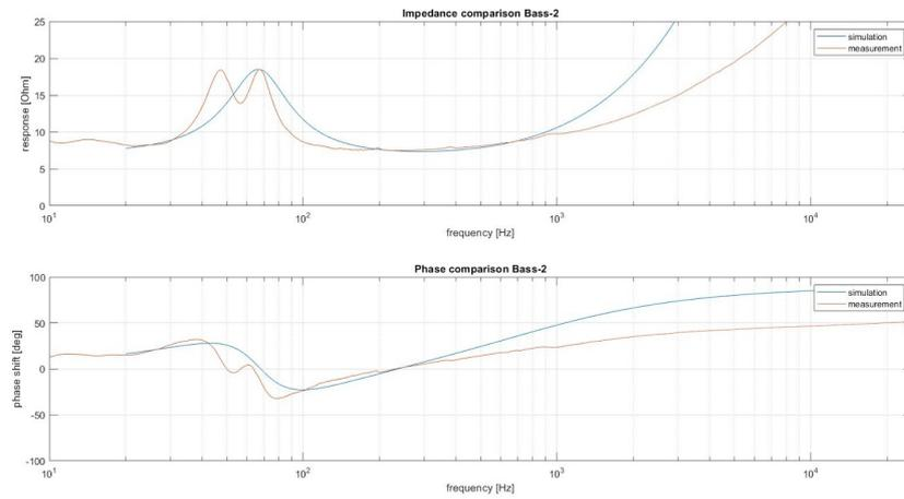
Figure 8.14: Comparison of measured and simulated impedance amplitude and phase of woofer 2
