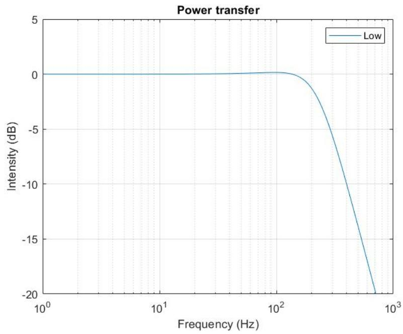
Figure 8.36: Low pass filter simulation
