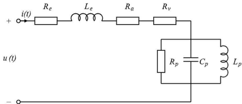
Figure 8.5: Impedance model for a speaker element.
