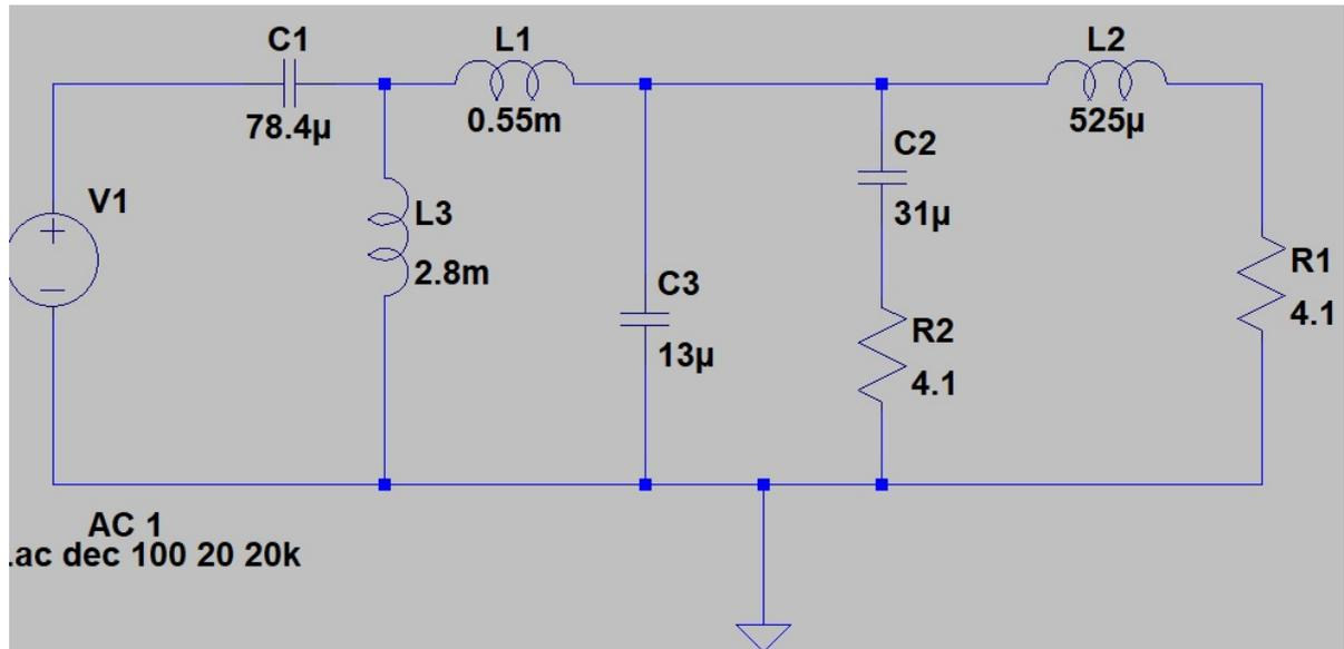
Figure 8.32: Band pass filter circuit
