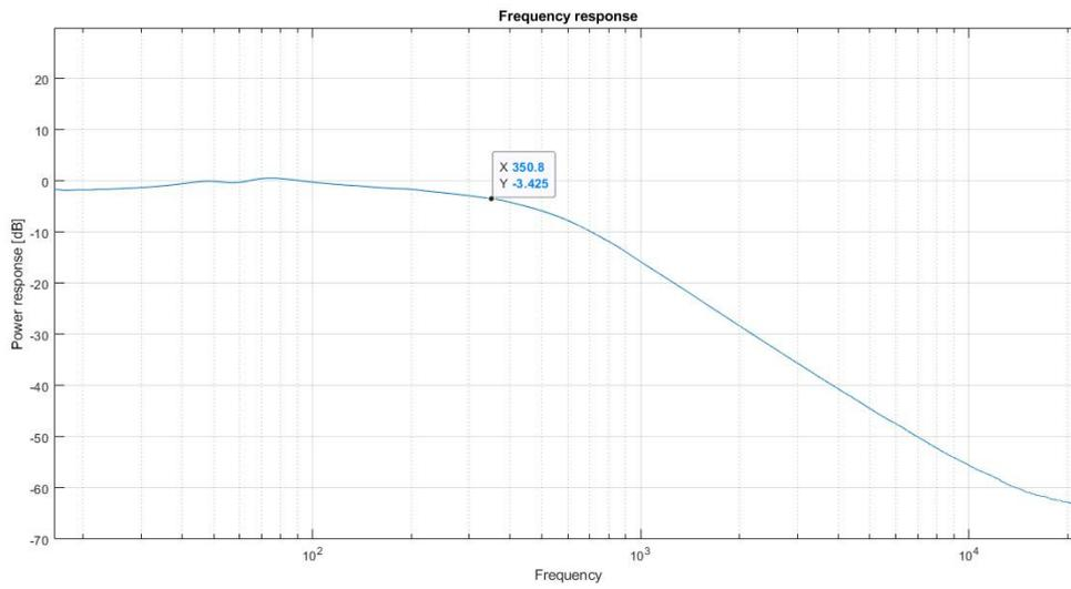
Figure 8.41: Electrical response Low-pass filter
