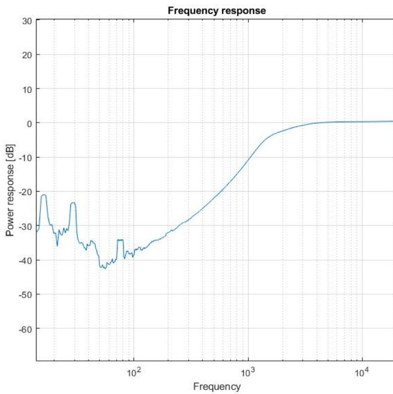
Figure 8.42: Electrical response high-pass filter
