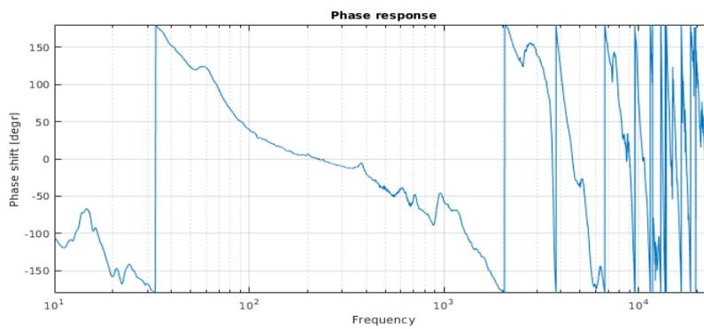
Figure 8.22: Acoustical phase response of woofer 2
